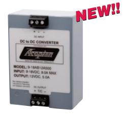
may be used in either polarity and floated up to 500 volts above the input. Optional output indicator (DC ON LED) and voltage adjust potentiometer are available for these units as well. Short circuit and thermal protection, and rugged encapsulated construction, assure years of reliable service.
