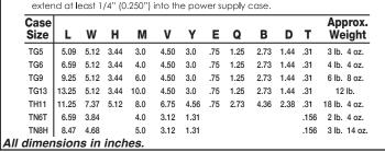
For **REAR MOUNTING of TN cases**, remove original 6-32 screws(4). These screws may then be used for mounting, provided they
