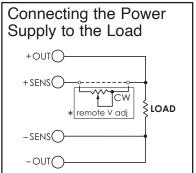
\*THE DOTTED LINE CONNECTION IS REQUIRED, unless remote voltage adjustment is used.
