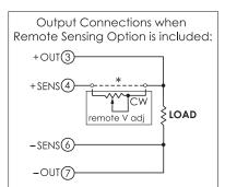
\*THE DOTTED LINE CONNECTION IS REQUIRED, unless remote voltage adjustment is used. If using remote adjustment, the remote pot should have the value in the table and the buill-in adjustment must be turned fully CCW.
