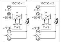
THE DOTTED LINE CONNECTIONS ARE REQUIRED, unless remote voltage adjustments are used. If using remote adjustments, the built-in adjustments must be turned fully CCW and the remote pots should have a value of 5K (0.5w).
