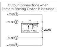
THE DOTTED LINE CONNECTION IS REQUIRED, unless remote valtage adjustment is used. If using remote adjustment, the built-in adjustment must be turned fully CCW and the remote pot should have a value of 5k (0.5w).
