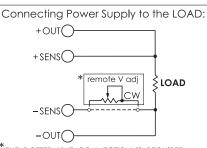
THE DOTTED LINE CONNECTION IS REQUIRED, unless remote voltage adjustment is used. A <u>potentiometer</u> OR <u>switched resistors</u> in the negative sense lead may be used to remotely program (adjust) the output voltage:
