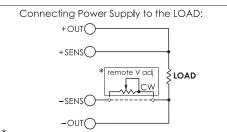
THE DOTTED LINE CONNECTION IS REQUIRED, unless remote voltage adjustment is used.
