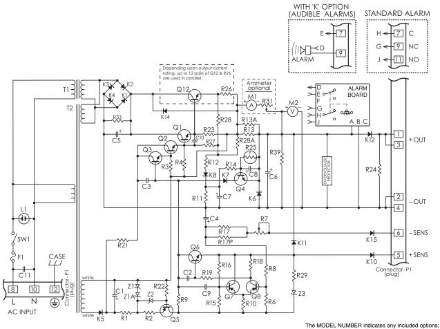
105 -125 VAC, 50-400Hz (Standard) 210-250 VAC, 50-400Hz (When model number ends in -230) The MODEL NUMBER indicates any included options; suffix A: ammeter suffix H: handles suffix K: audible alarm suffix –230: 230v input
